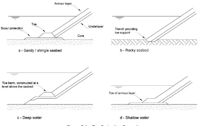
Figure 5.1: Toe Protection Examples Source: Ref. [9]
