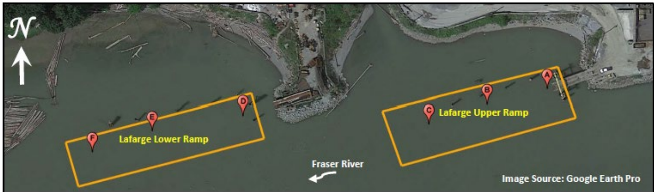
Figure 1. Approximate Dredging Footprint (orange polygons) fronting 2300 Rogers Avenue, Coquitlam, BC
