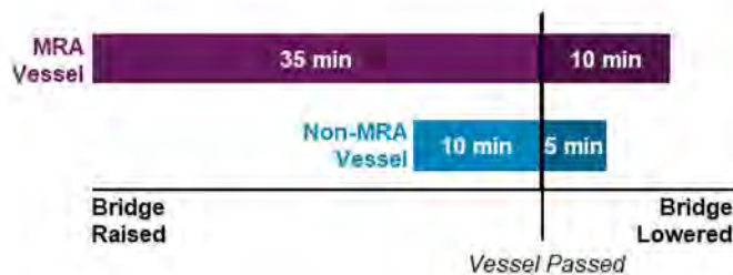
Figure 2-1 Durations for “Bridge Raised” to “Vessel Passed” and “Vessel Passed” to “Bridge Lowered”
