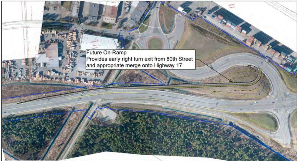
Figure 3-4: Highway 17 at 80 th Street Intersection Upgrade
