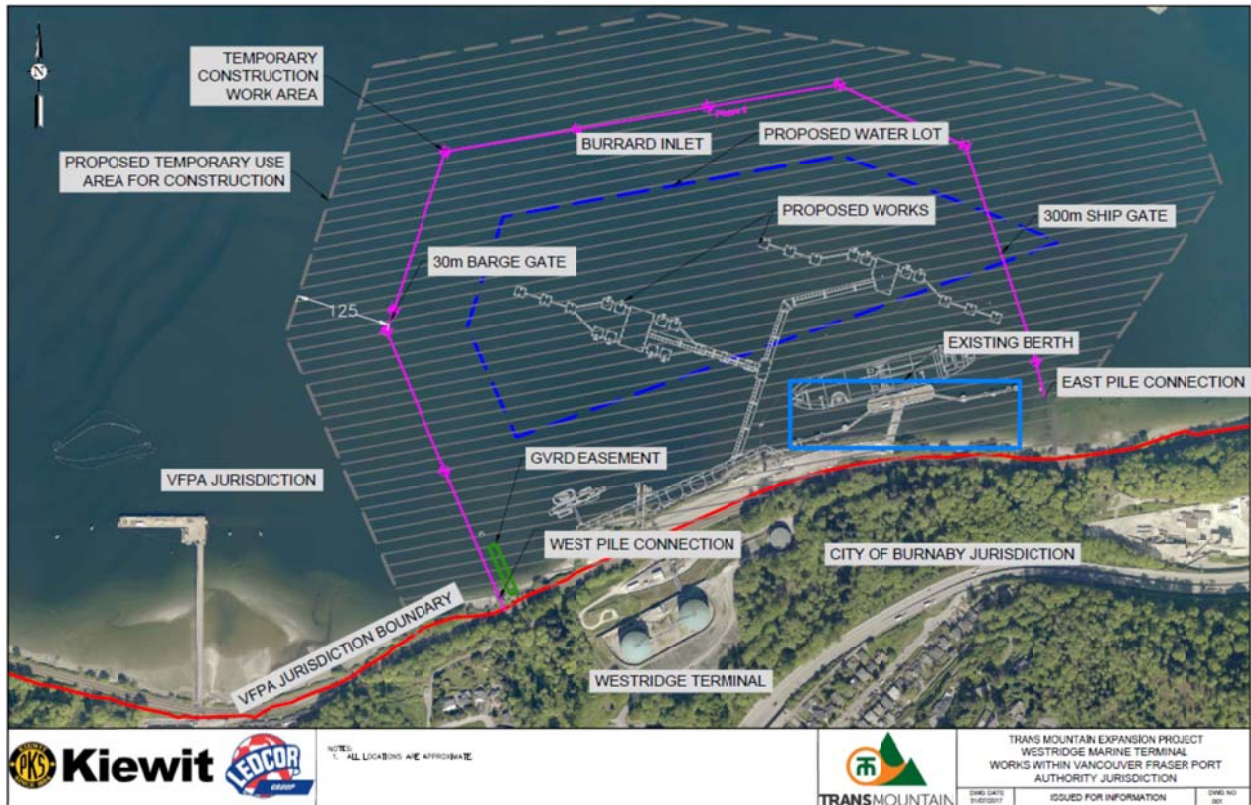
Figure 1: Proposed marine construction safety boom showing ship gate (concept only, actual layout might be different)
