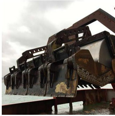
Pictured: One of the two 3.5 metres drag heads on the 309. These are connected to the dredging arms.
