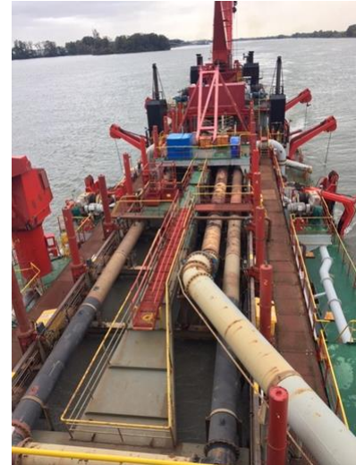
Pictured: View from the top of the dredging vessel where the suction pipes are visible.
