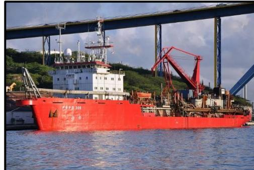
Trailing Suction Hopper Dredger FRPD 309 with hydraulically controlled drag head
