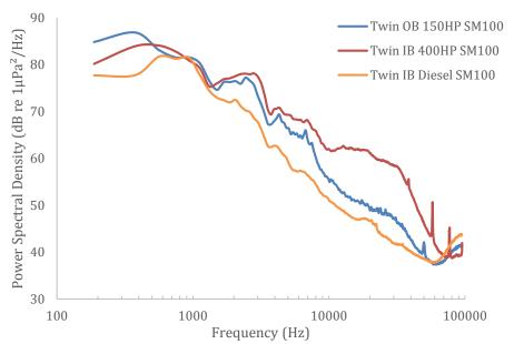
Figure 7 Power spectral density plots of the Hunt (2007) data for three different commercial whale watch boats. OB = outboard motor. IB = inboard motor. HP = horse power. SM = slow motoring (6 – 8 knots). 100 = range in meters between the slow motoring boat and the recording hydrophone.
