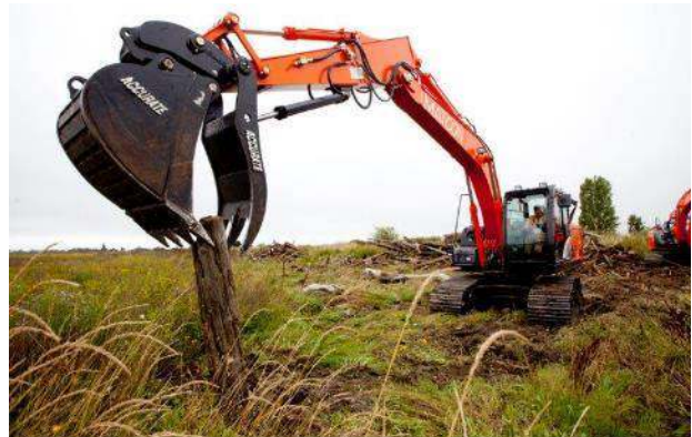
Photo 10. Installation of a vertical log to create a wildlife snag for a raptor perch (Photo Credit: W. Jans, September 2013).
