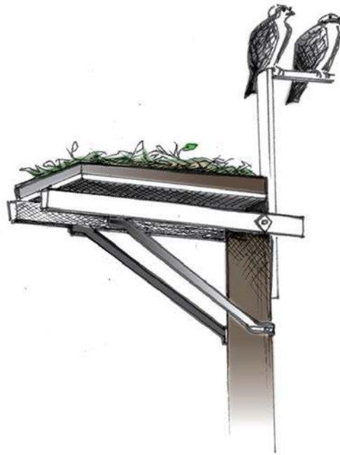
Preliminary rendering of osprey nesting platform design
