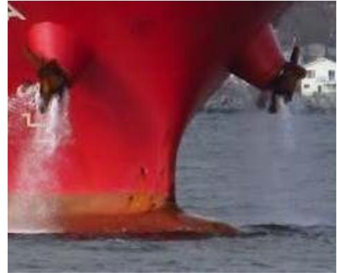
This is not to be confused with ballast water. People often confuse over-side discharges in English Bay. A deep-sea vessel is almost continuously suctioning seawater for various onboard systems. For example, aside from cleaning, seawater is also used to cool a vessel's main engine and generators. Once the water flows through the pipes and cools the equipment it is discharged.
