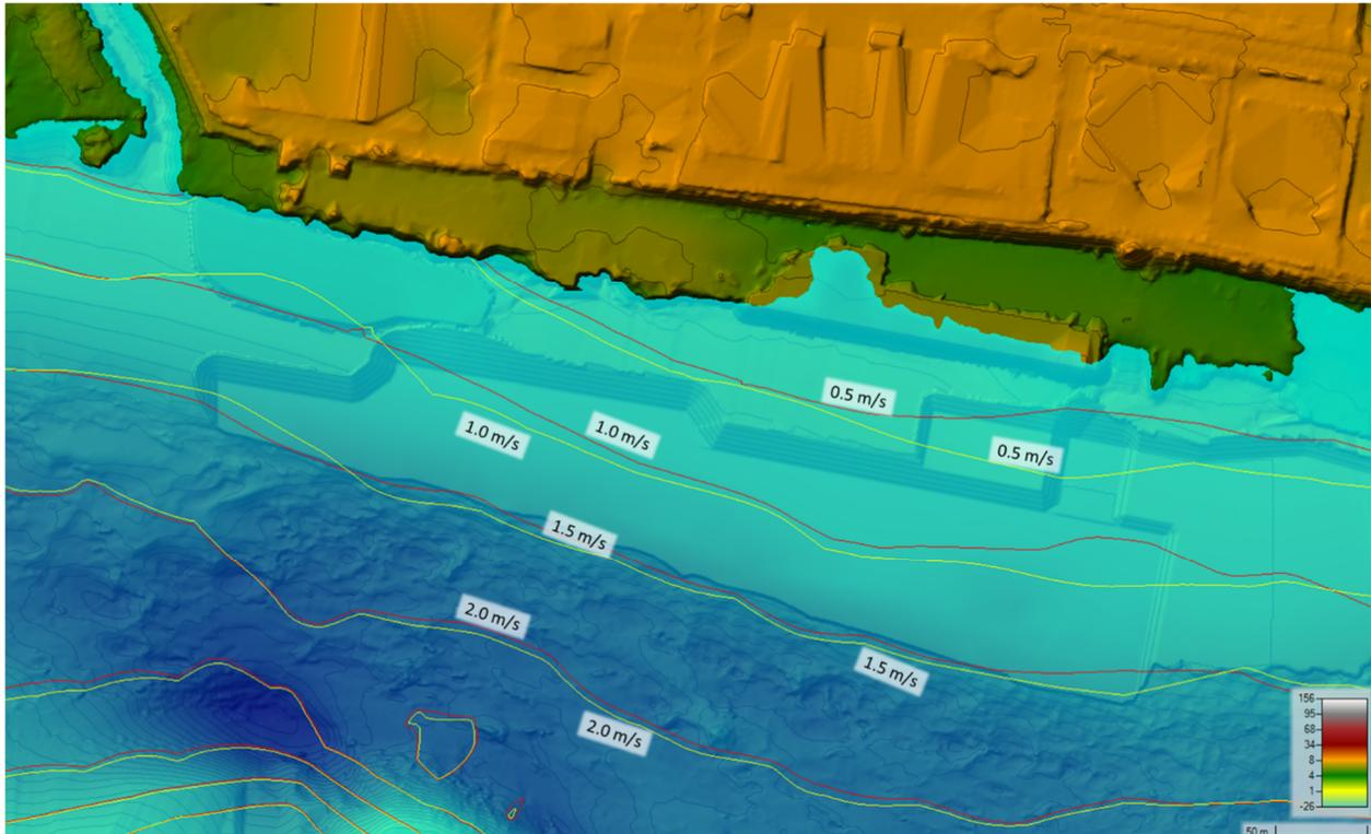
*Figure 1. Velocity contour for existing condition shown in red, and for proposed condition shown in yellow. Underlying terrain models shows dredging outline and habitat compensation bench.*
