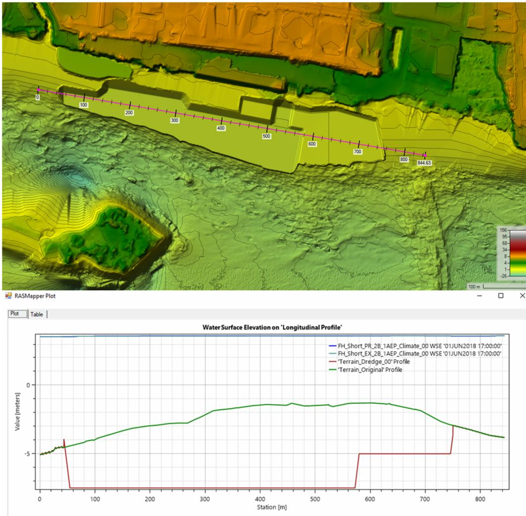
Figure 2. Profile line through dredging area (top). Existing ground (green line), proposed ground (red), and water surface (blue) along the profile line. Note that water surface lines for both existing and proposed conditions are on top of each other.
