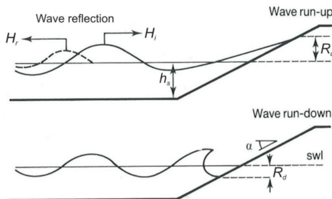
Exhibit 6.1: Hydraulic interactions related to waves and governing parameters (for wave run-up and wave-run down calculations).
