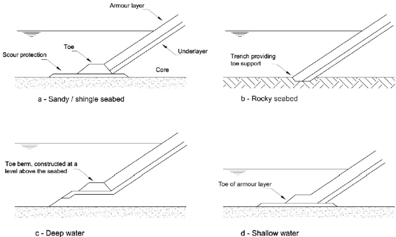
Figure 5.1: Toe Protection Examples
