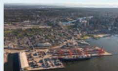
**Centerm Expansion Project and South Shore Access Project** These projects are being built to help meet anticipated near-term demand for containers shipped through the Port of Vancouver, and include a reconfiguration and expansion of the Centerm container terminal, a new overpass to remove road and rail conflicts, and changes to roadways and port lands access.
