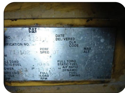
This engine data tag from a 1992 Caterpillar 14G motor grader shows the engine power rating is 200 hp or 149 kW.
