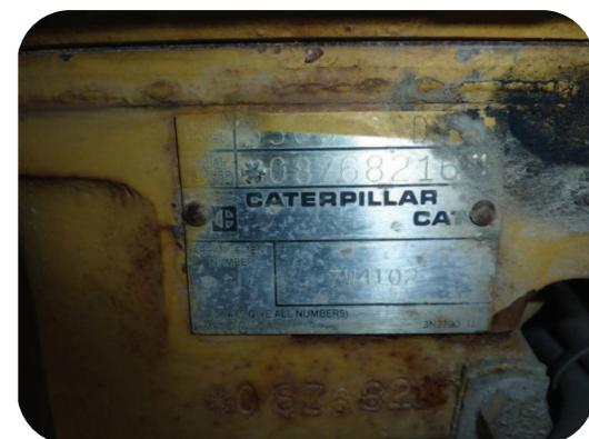
The engine serial number data plate from a 1992 Caterpillar 14G motor grader. The serial number reads 08Z68216
